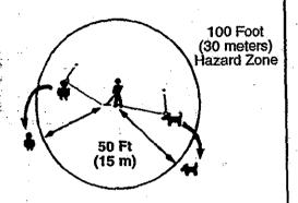
COASTING BLADE - THE BLADE CONTINUES TO SPIN AFTER THE ENGINE IS STOPPED OR THE THROTTLE IS RELEASED. THE COASTING BLADE CAN THRUST, THROW OBJECTS, OR SERIOUSLY CUT YOU IF ACCIDENTALLY TOUCHED. STOP THE BLADE BY LEAVING IT IN CONTACT WITH MATERIAL ALREADY CUT. USE THE "9 O'CLOCK" POSITION AS THE POINT OF CONTACT.
